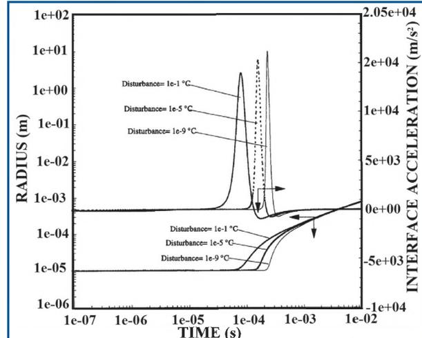
Fig. 3 Expected solution for the interface acceleration,  $\frac{d^2R}{dt^2}$ , of the coupled differential equations (5) and (6) for different initial temperature disturbances. Arrows point to the correct axis.
