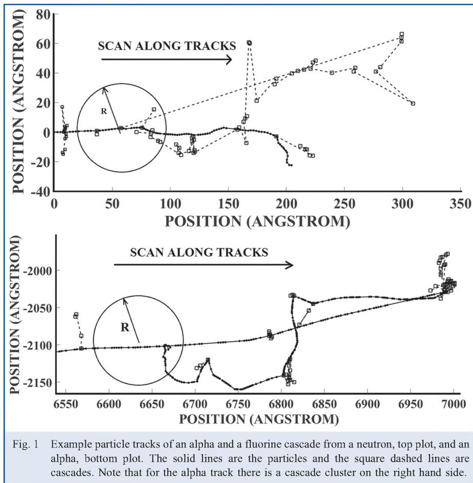
Fig. 1 Example particle tracks of an alpha and a fluorine cascade from a neutron, top plot, and an alpha, bottom plot. The solid lines are the particles and the square dashed lines are cascades. Note that for the alpha track there is a cascade cluster on the right hand side.
