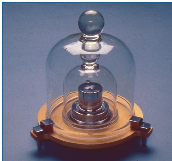
Fig. 2 Nested within several bell jars, rarely handled and stored in a controlled environment secure in a vault near Paris, *Le Grand K* is the artifact that presently defines the official SI unit of mass.
