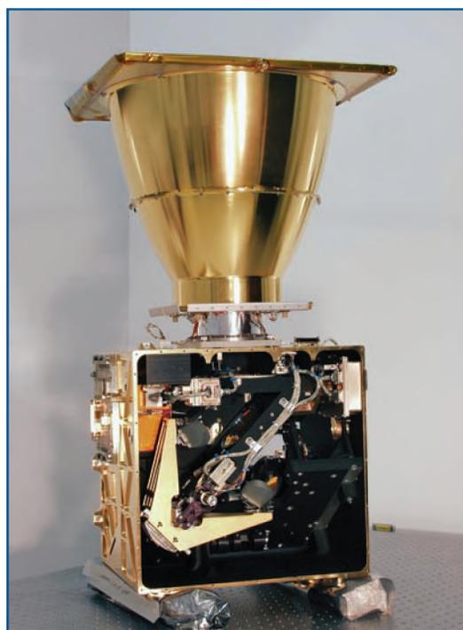
Fig. 1 Picture of the ACE-FTS instrument showing the interferometer arm and beam splitter configuration (from ABB Bomem). The cone located at the “top” of the instrument provides the passive cooler with protection from stray radiation from the Earth and the Sun.
