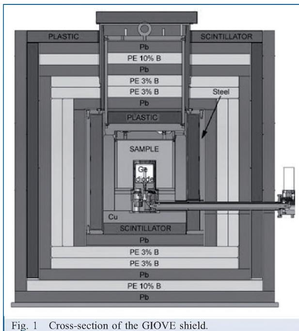
Fig. 1 Cross-section of the GIOVE shield.
