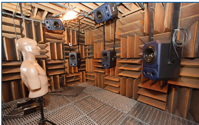
One of NRC's acoustic labs, an anechoic chamber built to absorb sound and eliminate echo, allowed NRC metrology experts to pioneer science-based methodologies still used today for measuring loudspeaker performance. (Circa 1980)
