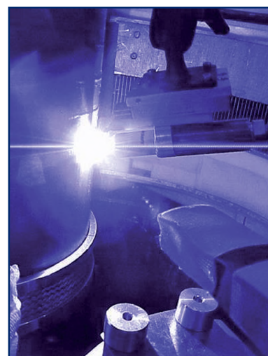
In-situ studies of welding on C2, the powder diffractometer.
