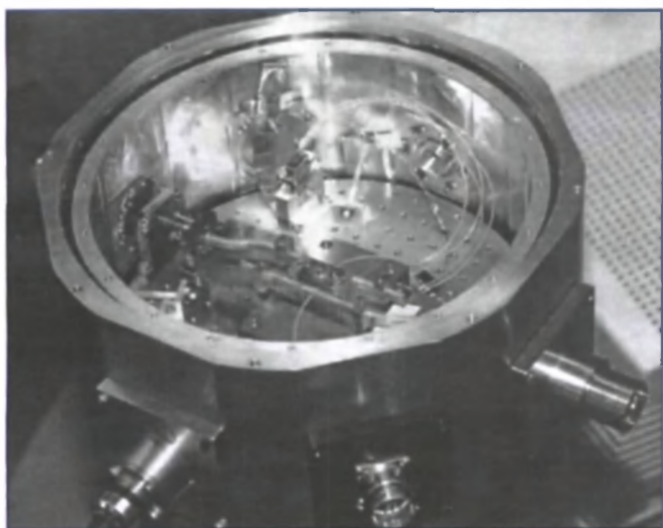
Fig. 1 A 75 GHz superconducting resonator system for cavity perturbation measurements.
