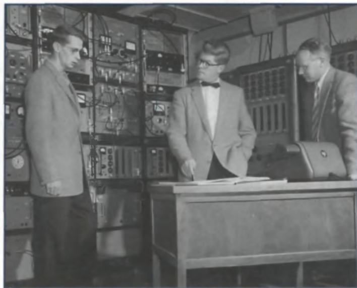
Fig. 1 Chalk River physicists (left to right) John Kuehner, Allan Bromley and Einar Almqvist in the experiment control room of the 3MV vertical Van de Graaff accelerator. The year is 1957 and in the background, on the right, can be seen relay racks each containing six channels of a Moody kicksorter (so called after its designer).
