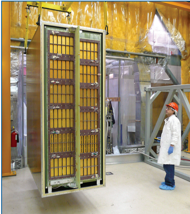
Fig. 2 Time projection chamber under construction in clean-room at TRIUMF under the watchful eye of Robert Henderson (TRIUMF).
