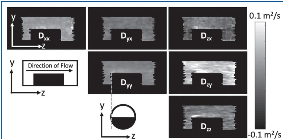
Fig. 3 The central slice of the eddy self diffusivity tensor with sketches of the pipe geometry.
