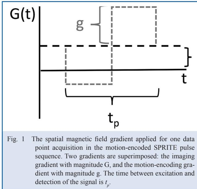
magnetic field gradients are superimposed. The constant gradient is known as the imaging gradient, and the bipolar gradient is known as the motion-encoding gradient. The time  $t_p$  represents the time between excitation of the sample via a radio-frequency pulse, and detection of the resulting signal.
