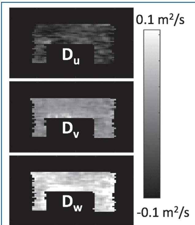
Fig. 4 The three eigenvalues of the eddy self diffusivity tensor in Fig. 3.
