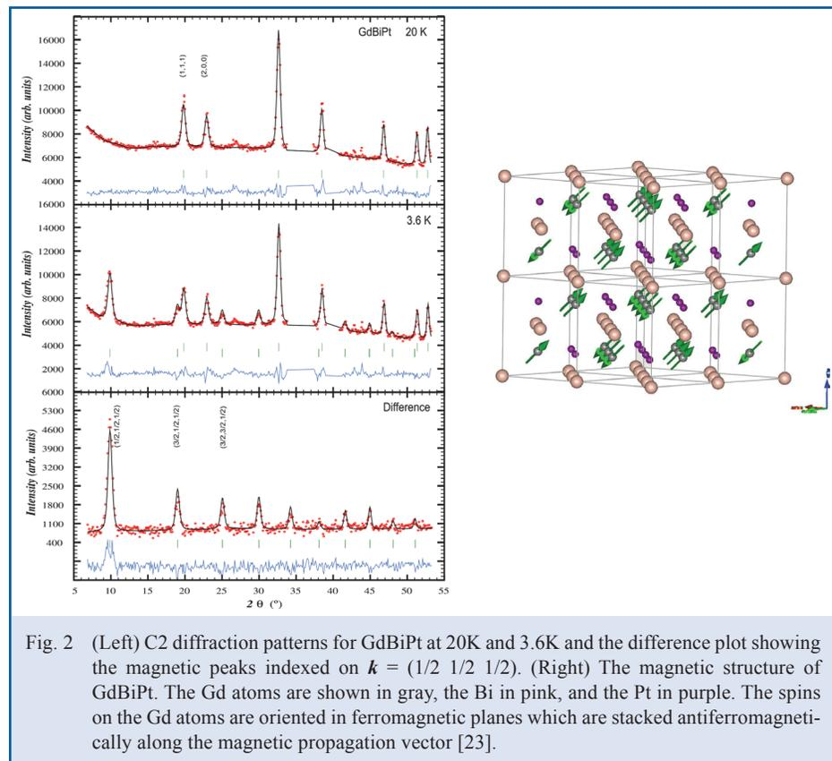
Fig. 2 (Left) C2 diffraction patterns for GdBiPt at 20K and 3.6K and the difference plot showing the magnetic peaks indexed on  $k = (1/2 \ 1/2 \ 1/2)$ . (Right) The magnetic structure of GdBiPt. The Gd atoms are shown in gray, the Bi in pink, and the Pt in purple. The spins on the Gd atoms are oriented in ferromagnetic planes which are stacked antiferromagnetically along the magnetic propagation vector [23].
