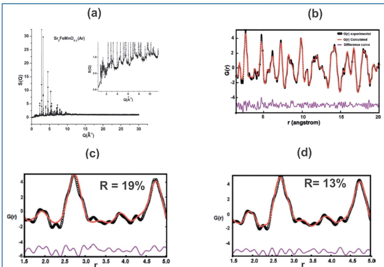
Fig. 13 (a) The  $S(Q)$  out to  $30\text{\AA}^{-1}$ . The inset shows broad features of the background upon which sharp Bragg peaks, consistent with Pm-3m symmetry, are superimposed. (b) The  $G(r)$  obtained by Fourier transform of  $S(Q)$ . (c) Fit of the  $G(r)$  to a cubic local model. (d) Fit of the  $G(r)$  to a brownmillerite local model.
