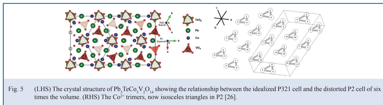
Fig. 5 (LHS) The crystal structure of  $\text{Pb}_3\text{TeCo}_3\text{V}_2\text{O}_{14}$  showing the relationship between the idealized  $P321$  cell and the distorted  $P2$  cell of six times the volume. (RHS) The  $\text{Co}^{2+}$  trimers, now isosceles triangles in  $P2$  [26].
