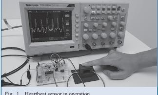
Fig. 1 Heartbeat sensor in operation.
