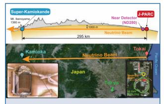
Fig. 1 Overview of the T2K experiment. A neutrino beam is produced at J-PARC (right inset), first measured at a near detector 280 m downstream, then propagates across Japan towards the Super-Kamiokande far detector (left inset) 295 km away.
