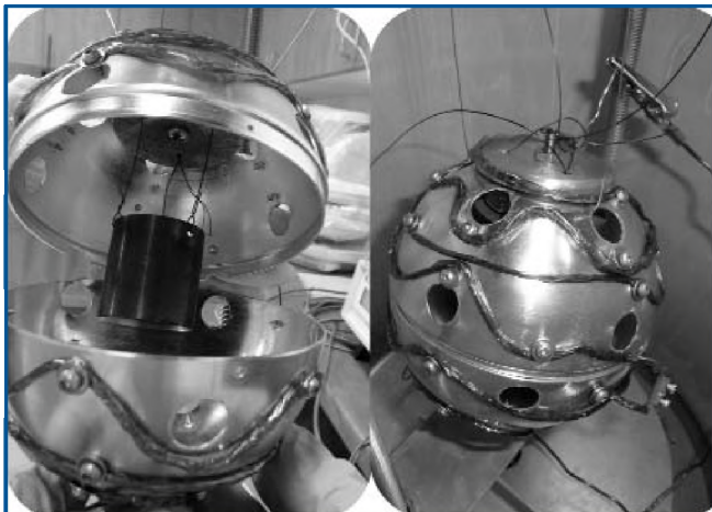
Fig. 2 The prototype large area TPB evaporation source.
