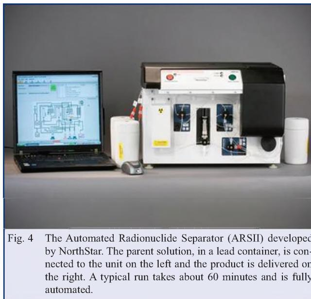
Fig. 4 The Automated Radionuclide Separator (ARSII) developed by NorthStar. The parent solution, in a lead container, is connected to the unit on the left and the product is delivered on the right. A typical run takes about 60 minutes and is fully automated.
