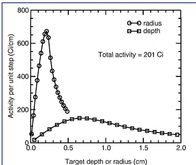
Fig. 7 Calculated activity for a 35 MeV, 100 kW, electron beam impinging on a cylindrical target of  $^{100}\text{Mo}$ , 1 cm in diameter and 2 cm long. The simulated irradiation period was 24 hours. The radial profile was calculated for cylindrical rings the length of the target while the depth profile was calculated for radial slices across the target.
