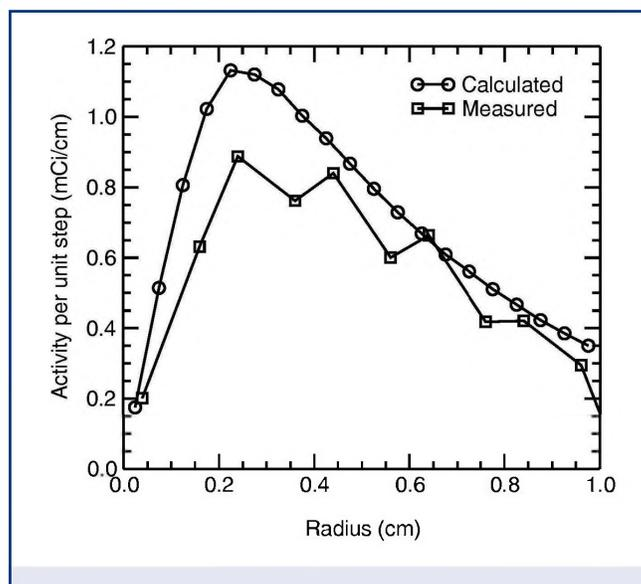
Fig. 6 Measured and calculated profiles of  $^{99}\text{Mo}$  activity for the upstream disk, irradiated as shown in Figure 5. The results are shown as activity per unit radial distance to better indicate the contribution of various parts of the disk to the total activity. There is little contribution from the centre of the disk because there is little material there, even though that is where the photon fluence rate is largest.
