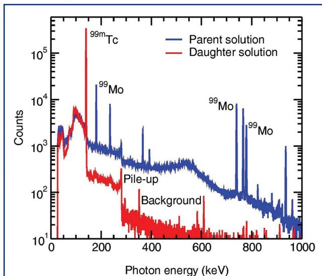
Fig. 8 Gamma-ray spectra of the parent solution (blue) presented to the ARSII separator and of the product solution (red). The edge at 280 keV is due to the pile-up of two  $^{99\text{m}}\text{Tc}$  lines.
