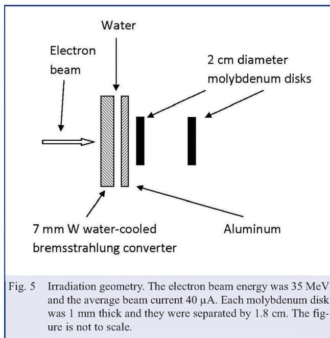
Fig. 5 Irradiation geometry. The electron beam energy was 35 MeV and the average beam current 40  $\mu\text{A}$ . Each molybdenum disk was 1 mm thick and they were separated by 1.8 cm. The figure is not to scale.
