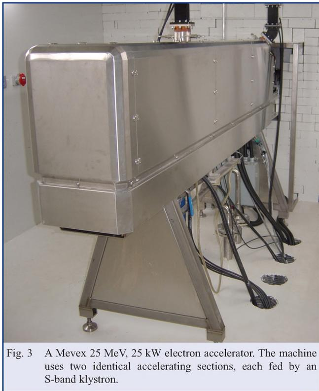
Fig. 3 A Mevex 25 MeV, 25 kW electron accelerator. The machine uses two identical accelerating sections, each fed by an S-band klystron.
