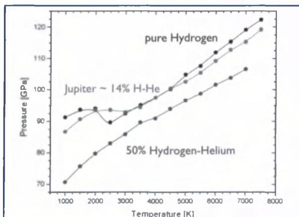
Fig. 1 Equation of state of hydrogen and hydrogen-helium mixtures at an electronic density corresponding to  $r_s = 1.60$ . The drop in pressure at  $\sim 2500\text{K}$  occurs as hydrogen molecules dissociate. The magnitude of this drop and the temperature at which it takes place is dependent on the fraction of helium present in the mixture.
