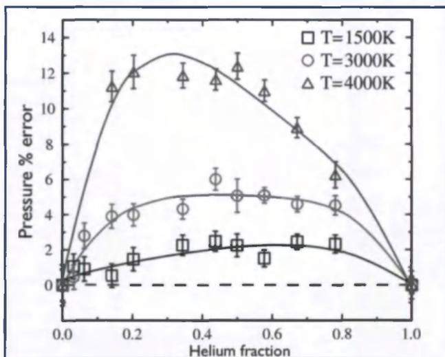
Fig. 2 The linear mixing approximation can be tested using our first principles data. A comparison is made between the pressure predicted from linear mixing (average of pure H and pure He EOS) and what we find in actual simulations of H-He mixtures.
