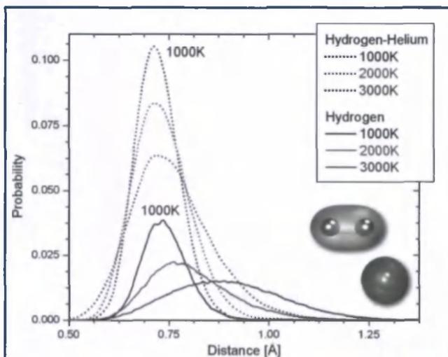
Fig. 3 Nearest neighbour distance distributions of hydrogen atoms for pure and mixed systems at the same electronic density ( $r_s = 1.60$ ). Based on the width of the distributions we see that the presence of helium results in stronger H-H bonds.
